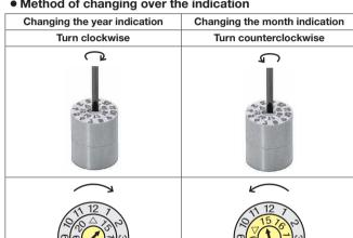
When the center part is turned clockwise, only the inside arrow rotates, enables the year to be changed. In the case of a date changeover type,
