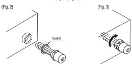
\*Confirm that there is no liquid leakage after tightening
