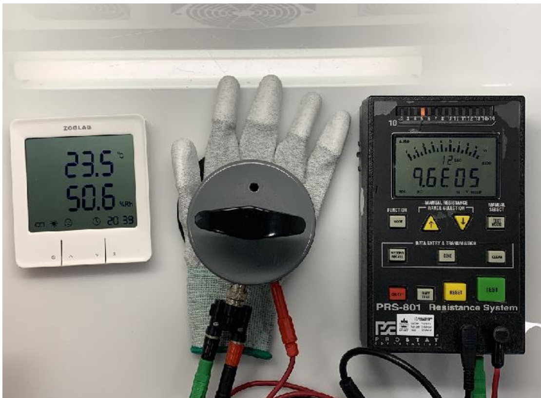
Figure 2: Surface Resistance Test (Outside)
