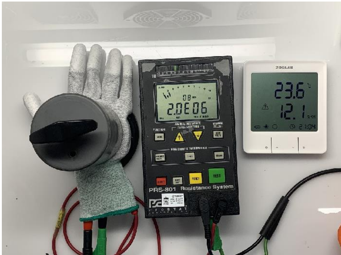
Figure 1: Surface Resistance Test (Inside)
