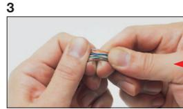
3 Straighten the disassembled cables. After that, cut the peeled sheath to 14 mm.
