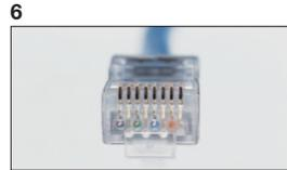
6 Confirm that all wires are fully inserted. Assembly is complete.
