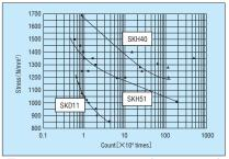
■ Fatigue strength of punching tools (rotating bending)
