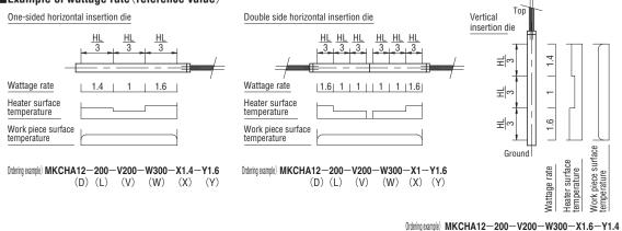
\* In the above wattage rate example, the wattage rate, heater surface temperature and surface temperature of the work piece are reference values.
