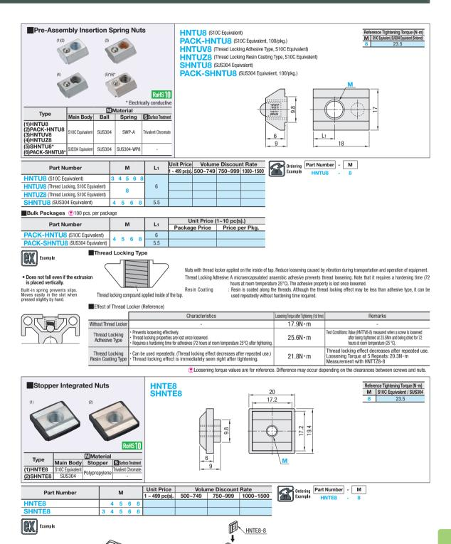
Integrated Pre-Assembly Insertion Nuts and Stoppers. The nuts do not slip off even if inserted into the vertically-placed extrusions
