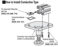
Conductive washers and toothed washers are not included with Conductive Type.
