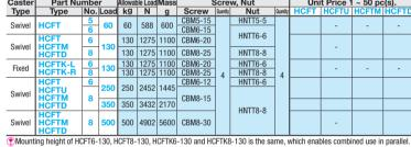
The stated allowable load is for the caster. Consider the allowable load of the leveling mount to be the same.
