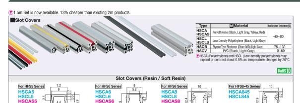
Slot covers are used in reverse as Plate Covers, HES5 can hold a 3mm plate, HES6, HES8 and HES8-45 can hold a 5mm plate. \*\* HSCL (soft resin) is made of softer material compared to HSCA (resin). Post assembly insertion is easy. (For details, see lower section of P.773.)
