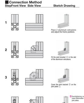
Tighten a hex socket head cap screw ③ to fix the plate. (Reference Tightening Torque: 15N • m)
