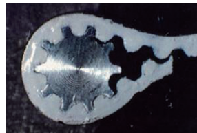
Static Backlash between the 2GT Type Belt and the Pulley (Number of Pulley Teeth: 20)
