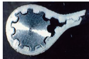
Static Backlash between the MXL Type Belt and the Pulley (Number of Pulley Teeth: 20)
