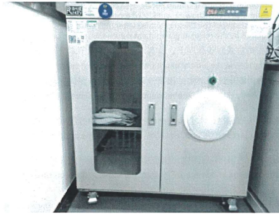
Low humidity drying Cabinets( Humidity:12.0%RH)
