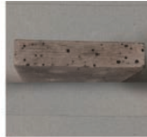
Blistering by heating
