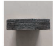
Delaminated by heating, weak pressure-bearing capacity
