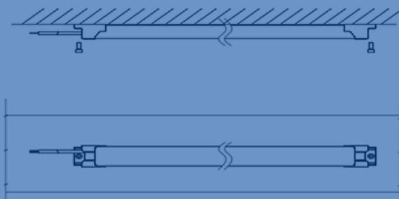
Mounting Method 1 Nut Installation
