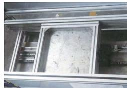
Test Conditions: Install the sample correctly on the durability tester, load 24.5KG in the drawer, make continuous pushing and pulling movement with a speed of 12 cycles/minute, observe the change of the sample and record the state of the product when the corresponding number of cycles is reached.
