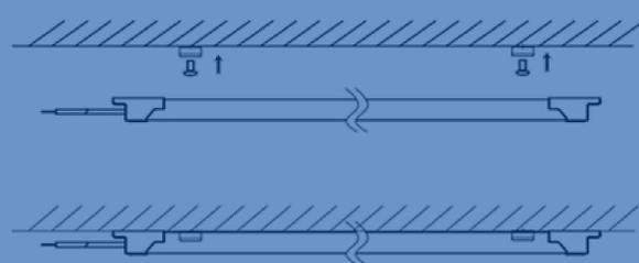
Mounting Method 2 Light Clip Installation
