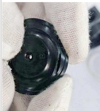
Damage and air leakage
