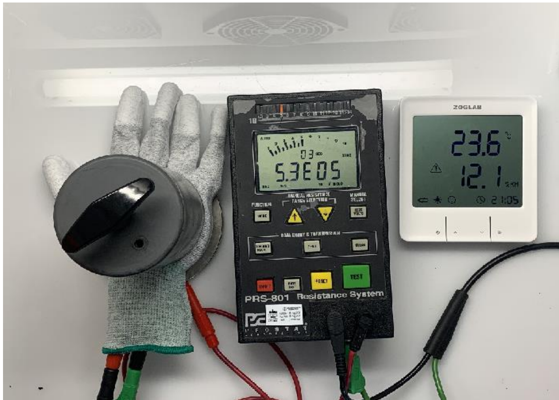
Figure 1: Volume Resistance Test (Inside)
