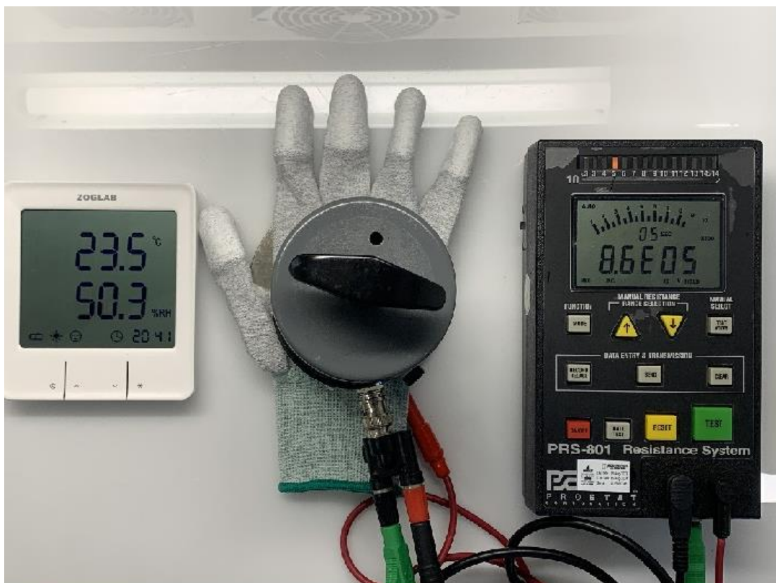
Figure 2: Volume Resistance Test (Outside)
